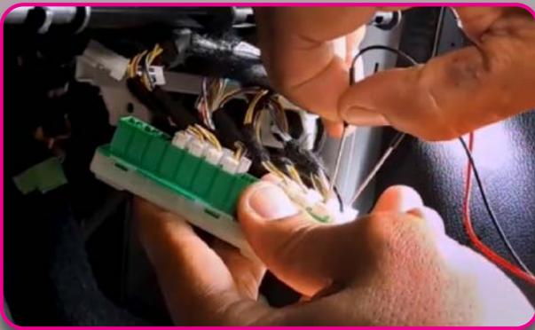
In this situation, connect the red pin into the green wire, and the black pin into the yellow wire.
